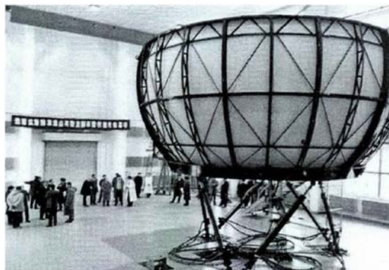
Figure 3 Six degrees of freedom driving simulator of Jilin University
